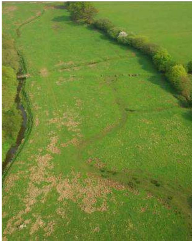
Aerial photo showing old river channel running through the middle of a floodplain, with a modern ditch or 'cut' draining water left). Restoring old river channels can help create better habitats for wildlife and more floodwater storage for people.
